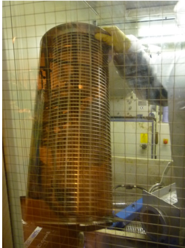
Fig. 13, Stainless steel filter representative of the type to be fogged at NNL's Preston facility.
